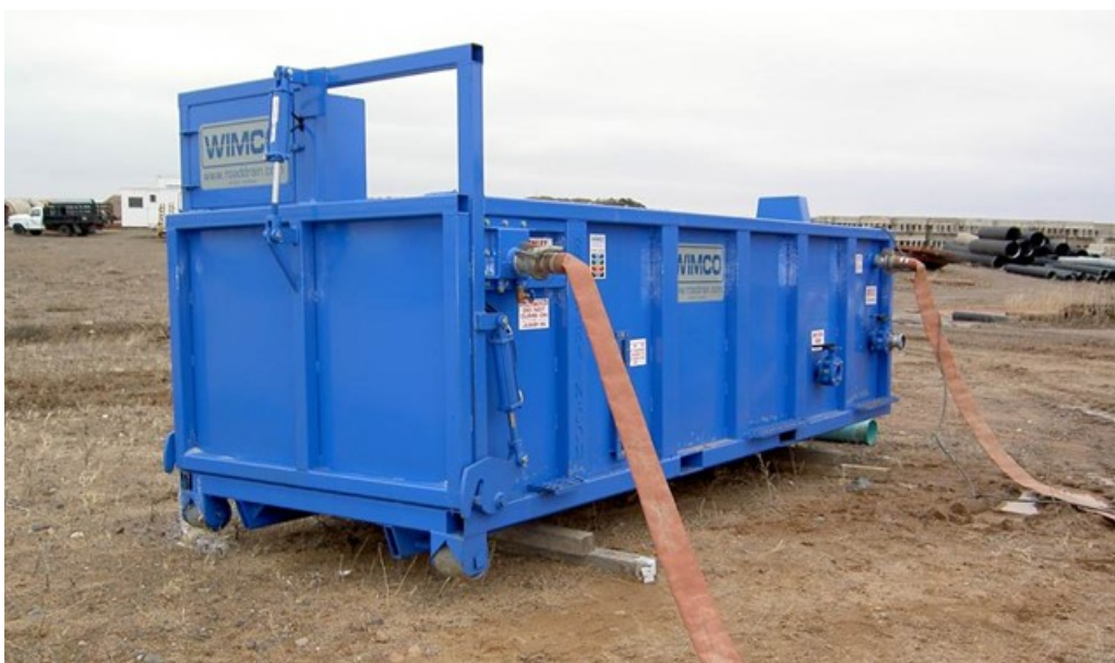
Photograph 4 Typical sediment control system
